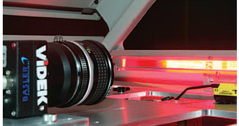
*Videk's VPS 9810 vision system placed inside the Bourg stacker, monitoring every page in real-time*
