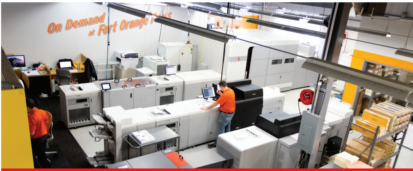
In addition to two Canon ColorStream series inkjet web presses, Fort Orange Press utilizes a Canon VarioPrint i300 full-color sheetfed inkjet press, Canon imagePRESS C10000VP full-color cutsheet toner presses, and Canon varioPRINT 6000 monochrome cutsheet toner presses.
