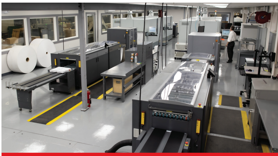
With a massive increase in the print volume and variable data complexity of absentee ballots in the 2020 election, Fort Orange Press relied heavily upon two Canon ColorStream inkjet web presses configured with inline trimming, perforating, and stacking capabilities to meet the individual time demands of its Boards of Elections customers.
