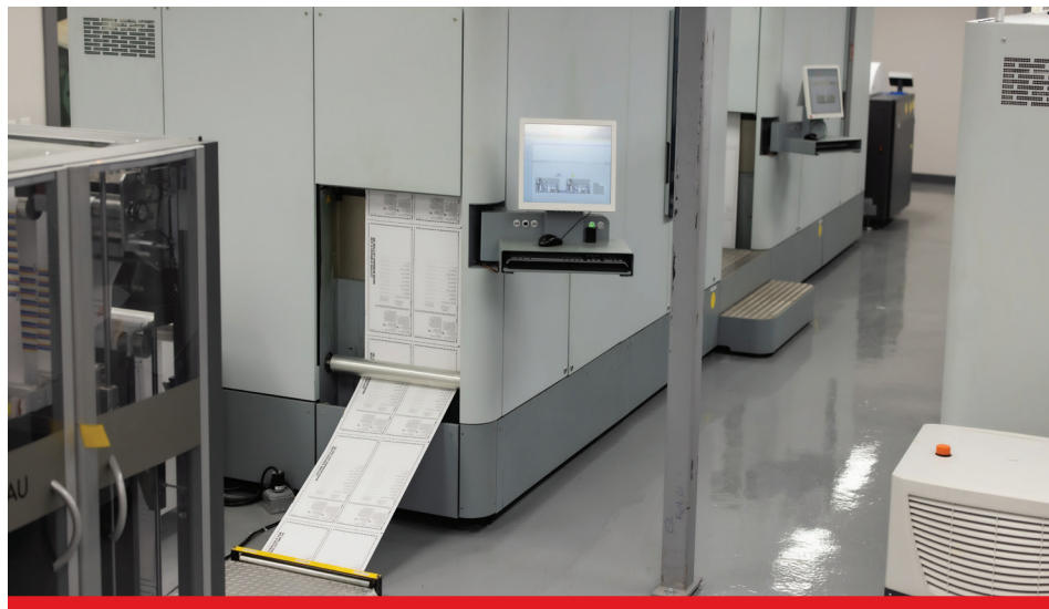
Considered the most reliable digital inkjet web press in the industry, Fort Orange Press uses two Canon ColorStream series presses, enjoying speeds of up to 417 linear feet per minute and 1,200 dpi perceived image quality.
